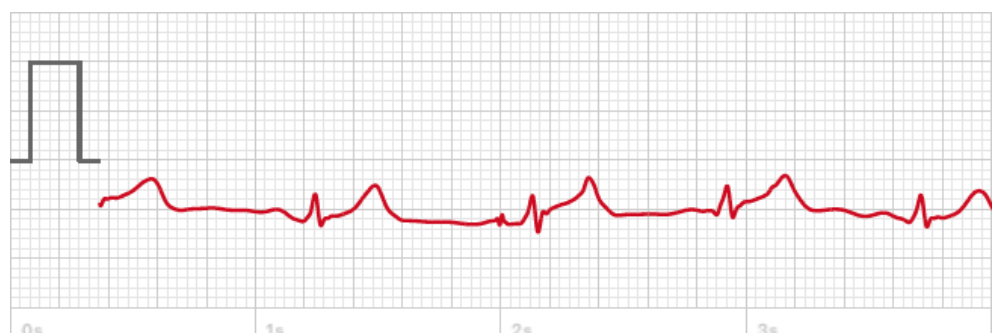
Figure 6.3: Example of a captured ECG signal with an optical heart sensor from a smart watch
